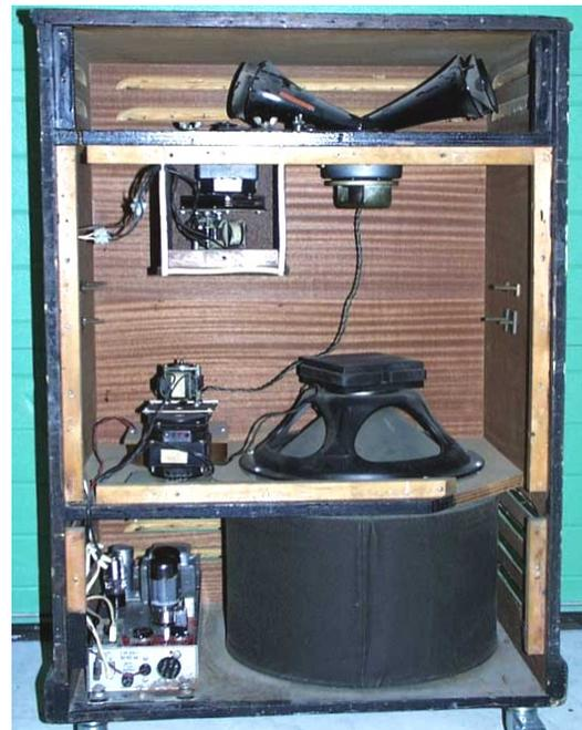
Fig. 1. The back side of a Leslie Model 147 speaker.
