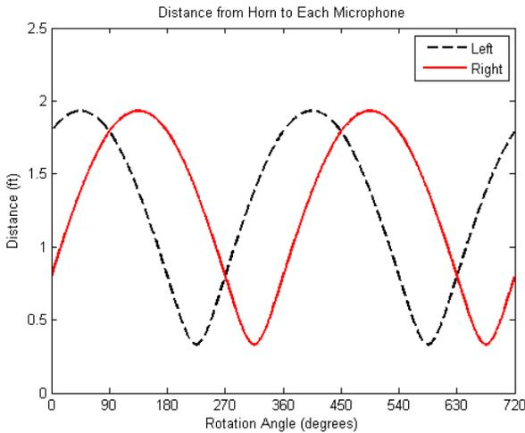
Fig. 4. Distance between the treble horn and each microphone, with respect to rotation angle.
