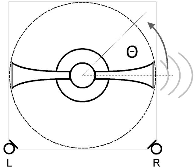
Fig. 3. Geometry of simulated rotating horn and microphones. Zero-degree axis points to the right.
