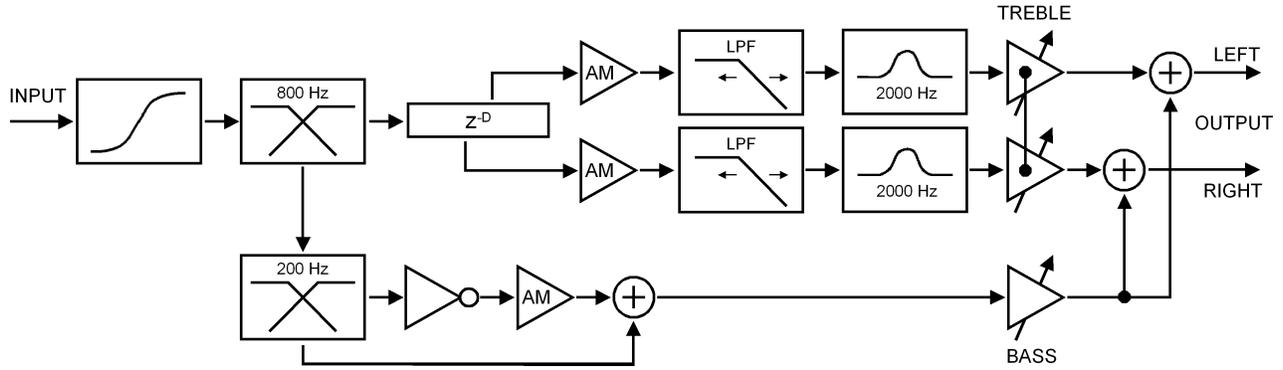
Fig. 2. Block diagram of the Rotary Circus algorithm.
