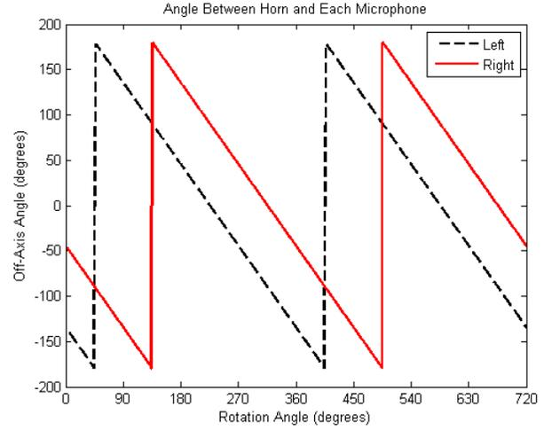
Fig. 5. Angle between treble horn and each microphone, with respect to rotation angle.
